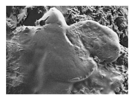
Ball-pen paste on laser printed document in the SUPRA<sup>TM</sup> 55. HV mode, 1 kV. No toner particle visible on the ball-pen paste is the proof of no falsification.
