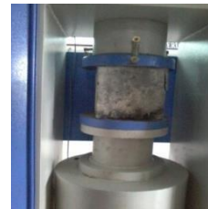
Figure Compressive strength test
